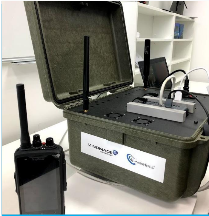
MC-NIB: a complete 4G or 5G network (RAN+Core) with MC applications (e.g., PTT)
