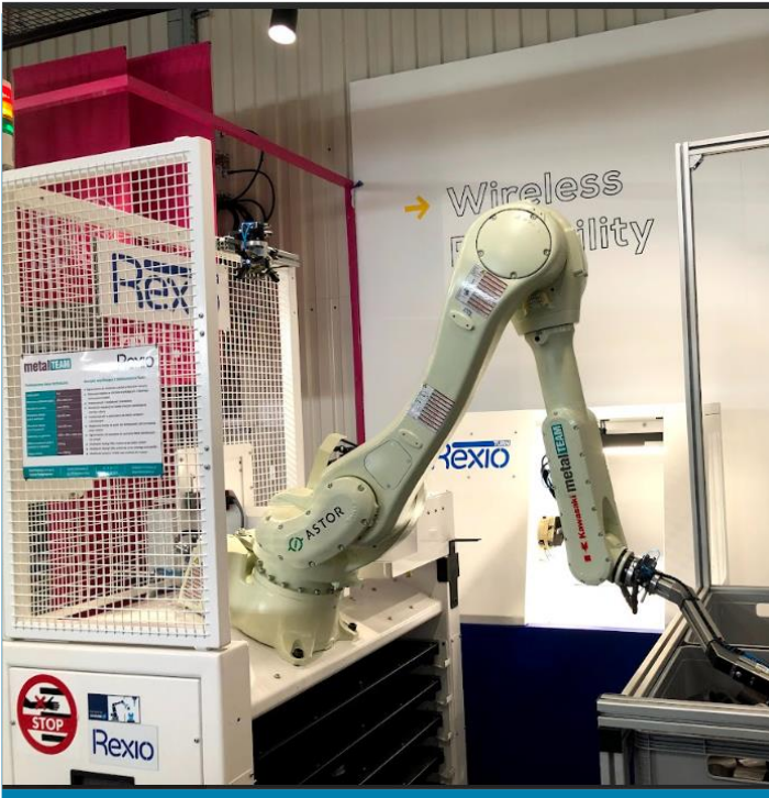
Kraków Astor company: 5G SA 3.6 GHz RAN (Core from T-Mobile), control of robots
